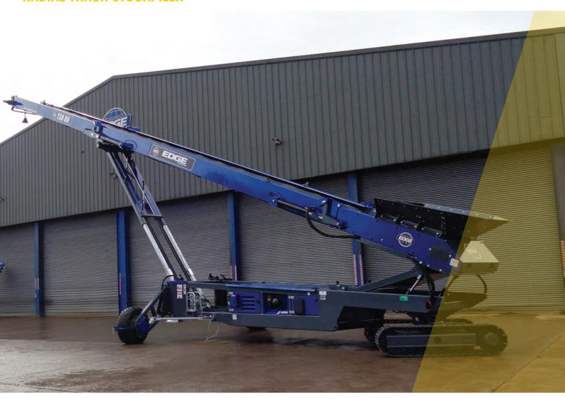
The EDGE TSR80 is a 80ft long tracked mounted conveyor with radial stockpiling functionality. The core design principal for the TSR80 has been to provide customers with an easily transported stacker that can be moved nationally and internationally with minimal fuss or cost. Designed to fit into a 40ft high cube container, with only small assemblies to be refitted upon arrival thanks to its' simple track in, track out philosophy.
