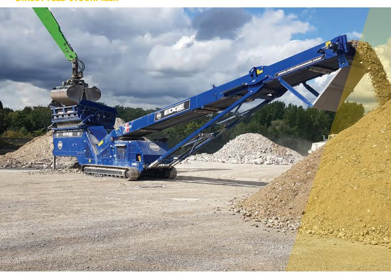
EDGE Innovate's range of Feeder Stackers have the ability to handle a wide range of applications and capacity requirements. Available with discharge conveyors from 30ft to 90ft, various chassis formats, power-source options and infinite number of add on options such as a two deck vibrating live head, overband magnet, wireless remote functionality and radio reject grid. The Feeder Stacker range is arguably EDGE Innovate's most versatile product.
