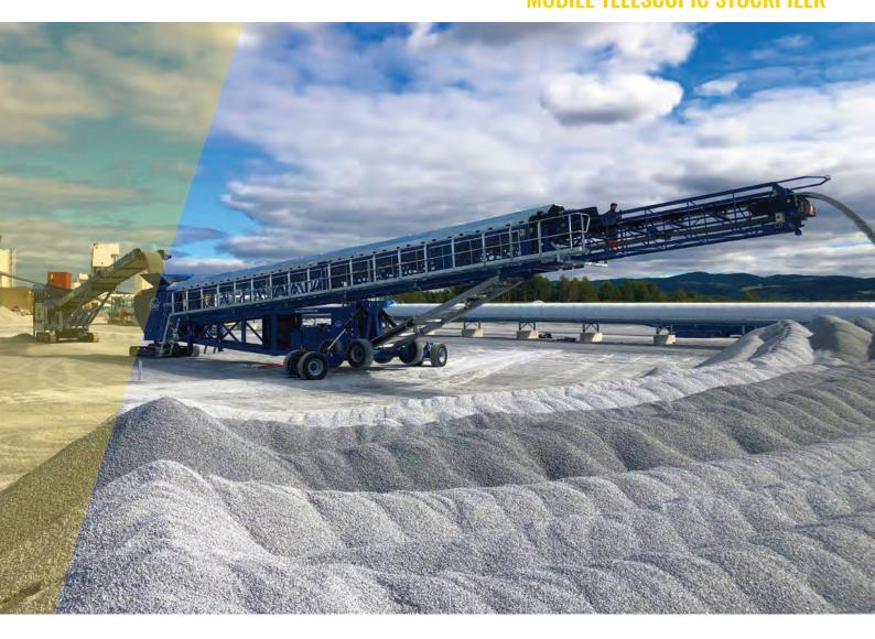
EDGE Innovate's MTS140 is a mobile mounted 140ft (42.2m) long telescopic stockpiler. It offers operators the most cost effective bulk material handling solution on the market. The MTS140 allows operators to achieve maximum stockpile capacity using a robust, fully automated stockpiling solution that eliminates the doubling handling of material and maintains high quality material via the creation of windrow stockpiles.
