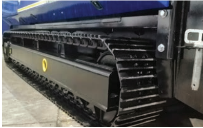
Tracked Mounted - Fully tracked for on-site manoeuvrability
