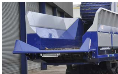
Hydraulic Raise / Lower Feeder Tail Door.
