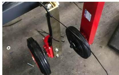
Belt Scale - fitted to collection conveyor.
