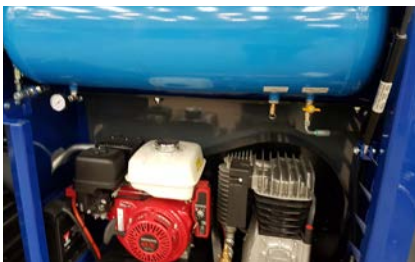
Air Compressor - multiple air line inlet-ports provided.
