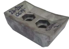
Fine Shredding Tool - the sharp edge tool allows for the creation of finer particles.
